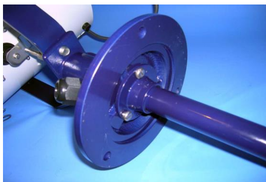
7. Fasten the Under Deck mechanism Using the 3 off M6 x 16 screws and spring washers
