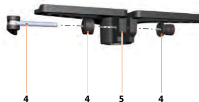
Fig. 61: Quick clamp and clamping unit control triangle
