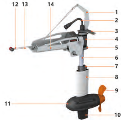
Fig. 51: Overview of Ultralight 1103AC components
